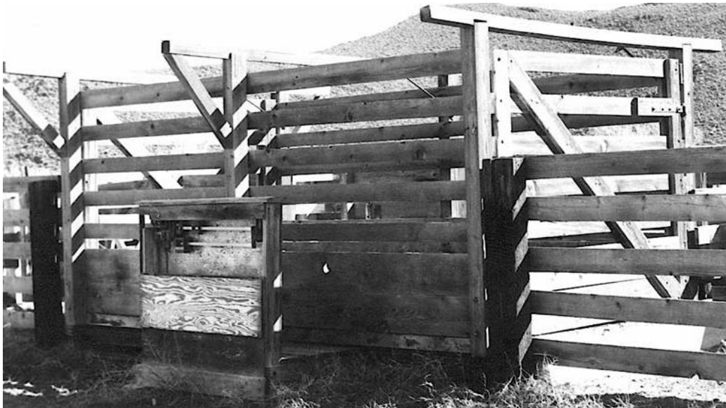
LIVESTOCK SCALE with WOOD CAGE
